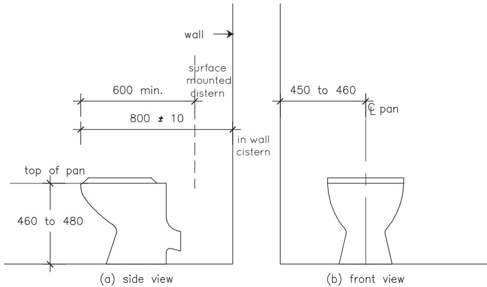
note: for the purpose of dimensioning, the front of the wc pan has been used as the datum plane
